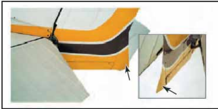
Figure 4-18. A ground-adjustable tab is used on the rudder of many small airplanes to correct for a tendency to fly with the fuselage slightly misaligned with the relative wind.
