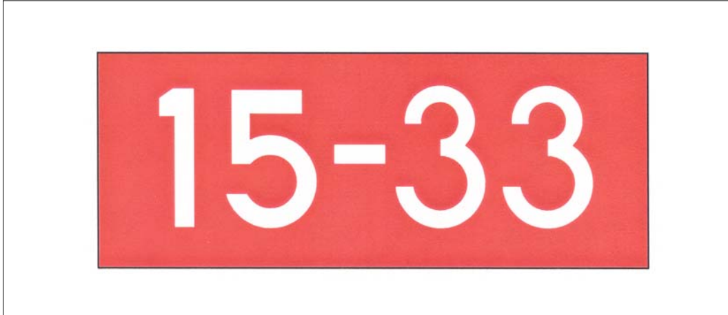
FIG 2-3-24 Runway Holding Position Sign
