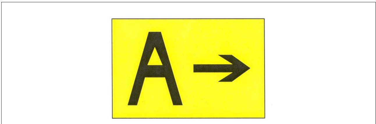
FIG 2-3-36 Direction Sign for Runway Exit
