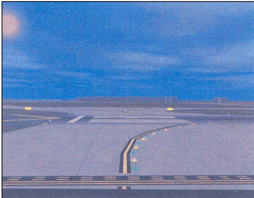
FIG 2-1-12 Taxiway Lead-On Light Configuration
