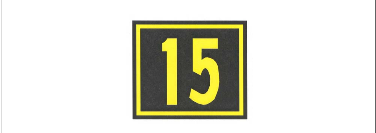
FIG 2-3-32 Runway Location Sign
